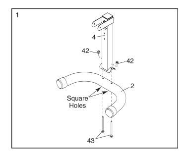
Orient the Rear Stabilizer (3) so that the square holes are on the side shown. Attach the Rear Stabilizer to the Frame (1) with two M10 x 90mm Carriage Bolts (43) and two M10 Nylon Locknuts (42). Do not tighten the Nylon Locknuts yet.
